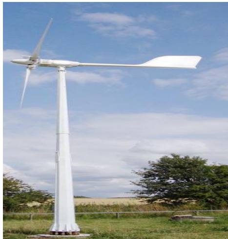
4.9 Kw wind turbine on an 8m pole
